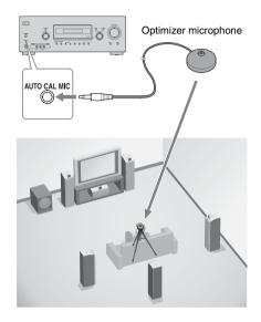
Connect the supplied optimizer microphone to the AUTO CAL MIC jack.
